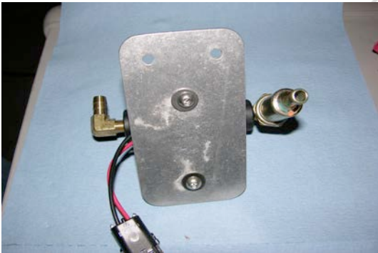
Mount the pump to the plate in the position shown.
