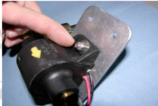
When mounting be sure to mount the pump, mount bolts with the nuts facing the pump as shown.
